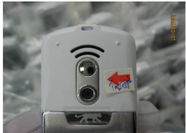
Missing protective film on camera
