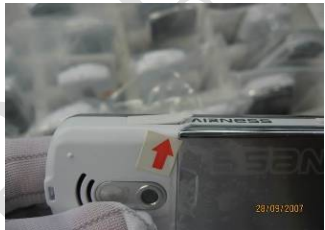
Slightly turn up of USB socket cover
