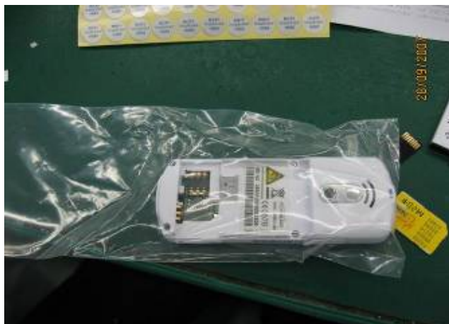
Missing battery cover
