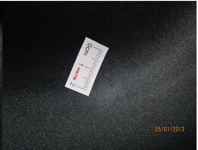
defect-item-810404-poor painting on inner surface(ma)-1
