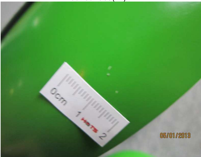
defect-item-810406- scratched mark on out-surface(mi)-3
