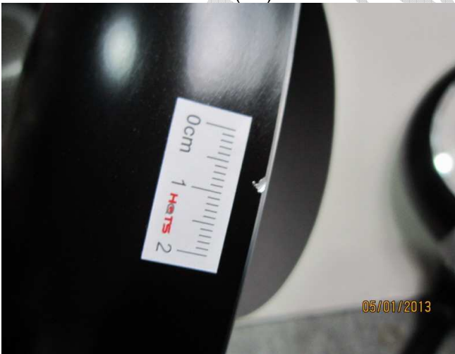
defect-item-810404-scratched mark on out-surface(mi)-2
