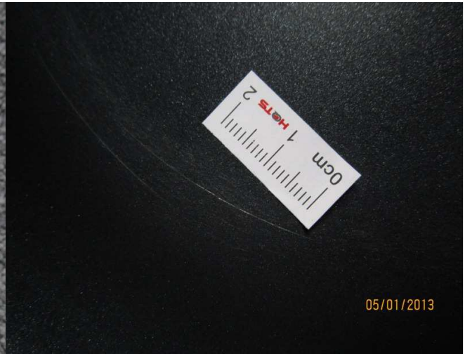
defect-item-810407-scratched mark on inner surface(ma)
