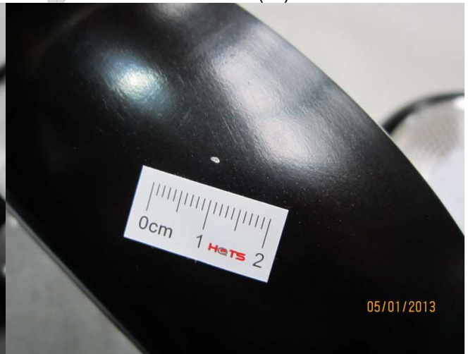
defect-item-810404-poor painting on out-surface(mi)
