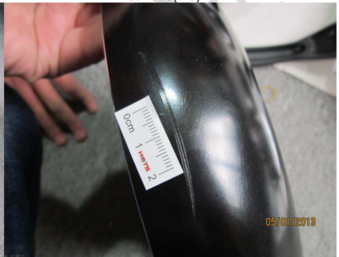
defect-item-810404-scratched mark on out-surface(mi)-1
