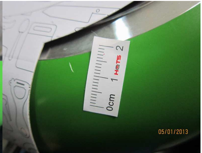
defect-item-810406- scratched mark on out-surface(mi)-2
