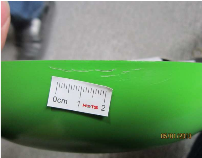
defect-item-810406- scratched mark on out-surface(mi)-1
