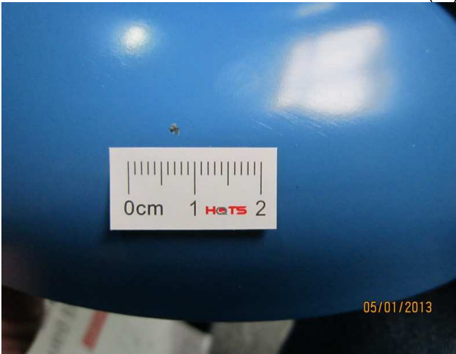
defect-item-810405-poor painting on out-surface(mi)-2 defect-item-810406-bottom-edge wasn't smooth(ma)
