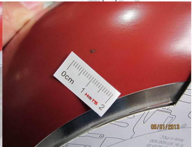
defect-item-810407-poor painting on out-surface(mi)-2
