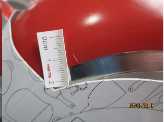
defect-item-810407-scratched mark on out-surface(mi)
