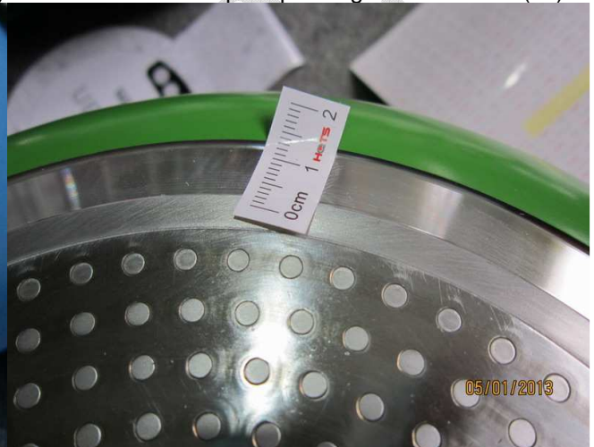
defect-item-810405-poor painting on out-surface(mi)-2 defect-item-810406-bottom-edge wasn't smooth(ma)
