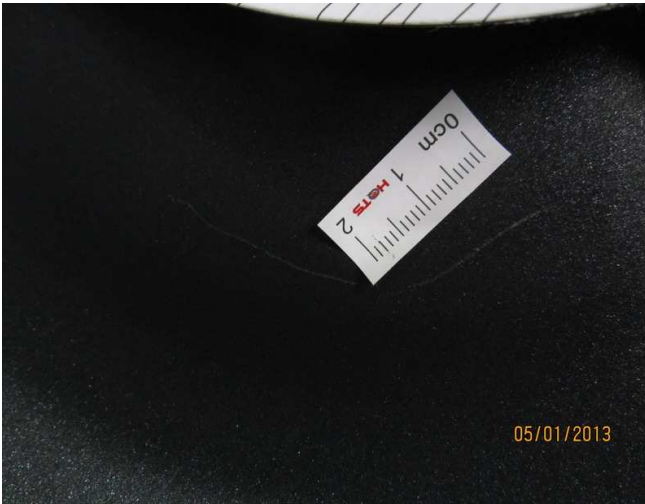
defect-item-810404-scratched mark on inner surface(ma)
