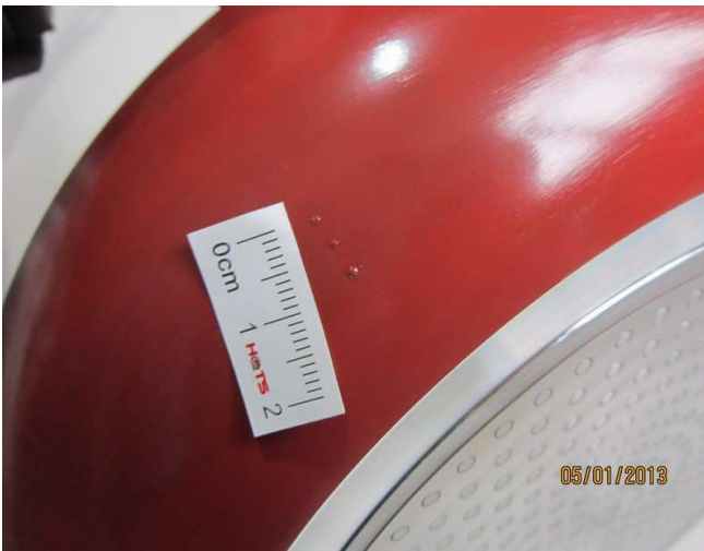
defect-item-810407-poor painting on out-surface(mi)-1
