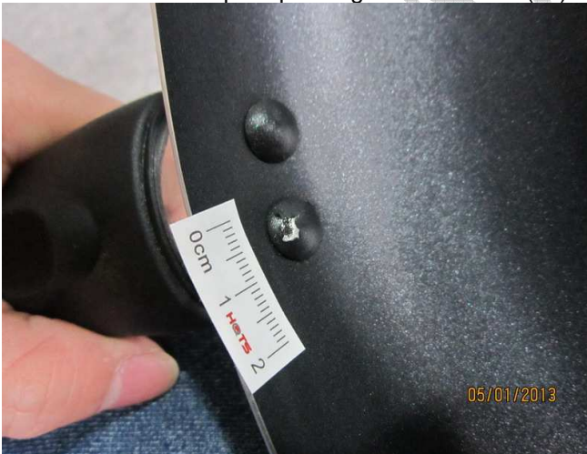
defect-item-810406-painting was peeled off on inner surface(ma)-1
