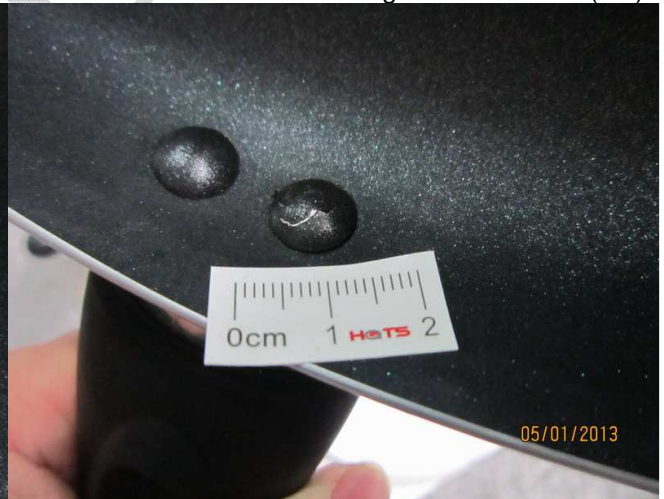
defect-item-810406-painting was peeled off on inner surface(ma)-2
