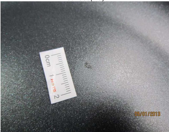
defect-item-810404-poor painting on inner surface(ma)-2
